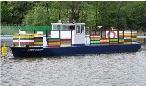
Figure 2 Manned model of ULCS
