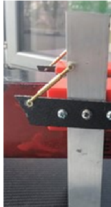
Figure 6 Regulation system of the front foil angle of attack
